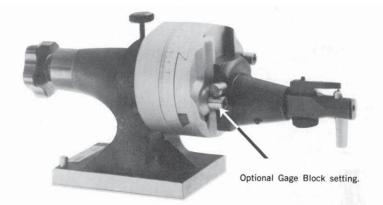
**ANY WHEEL FORM.** The grinding wheel may be dressed to any desired form — any combination of tangents and/or radii; either convex or concave.
